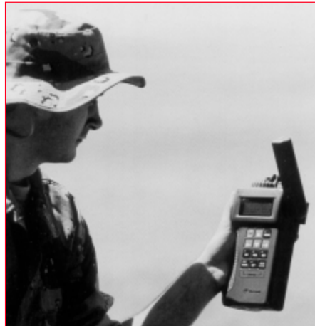
A military handheld GPS receiver (courtesy Rockwell)
