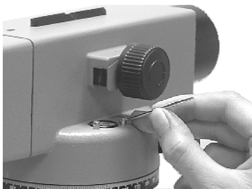
Fig.5 Adjusting the circular bubble.
